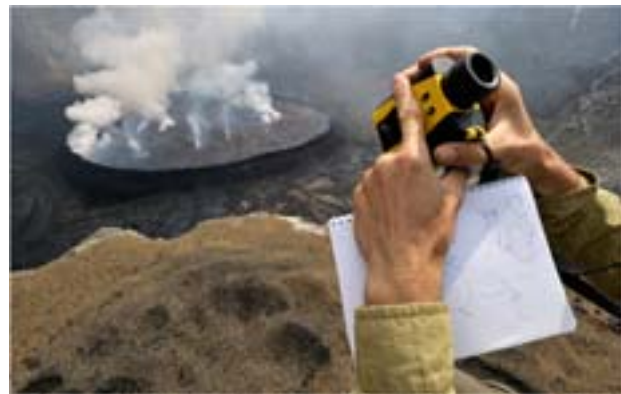
Using a laser telemeter, a member measures the changing size of the lava lake.
